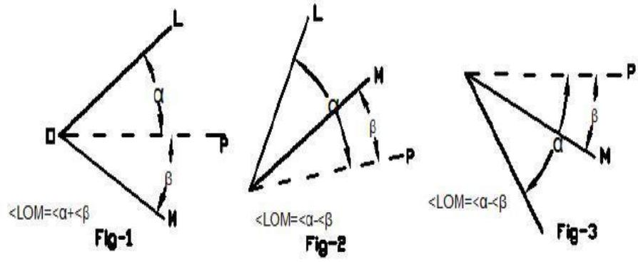
To measure the angle between two points L and M proceed as follows:
